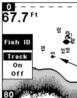
Fish ID menu and symbol with FishTrack on. The fish is 44 feet deep.
