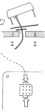
The plastic clip must be pressed in to pull out the plug contact.
